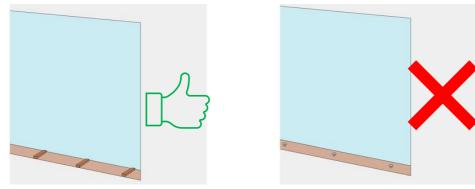
3. Attach the window using wood screws. Remember to use installation wedges!
